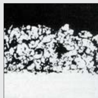
Microporous titanium Plasmapore® surface.
