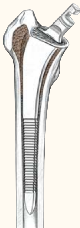
A-osteoprofiler with proximal compression surfaces
